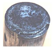
head gasket leak. In most cases the top of the cylinder and the face of the cylinder head must be resurfaced when a leak occurs. Most mx bikes have head stays mounting the head to the frame. Over time the head can become warped near the head stay mounting tab, because of the forces transferred through the frame from the top shock mount. It's important to check for warpage of the head every time you rebuild the top end.
